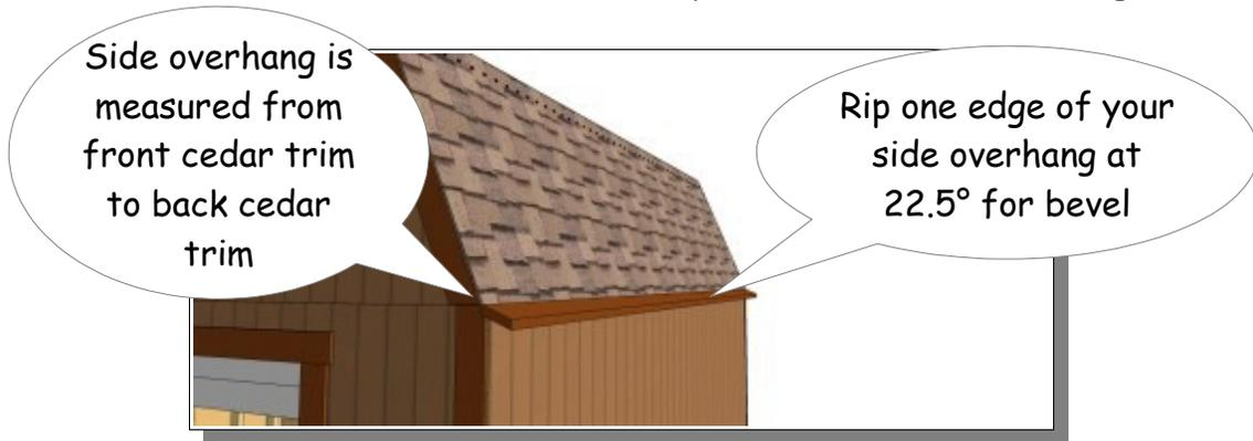
Now nail on the side overhang just underneath the bottom edge of the roof panel, and nail into the wall joists just behind the side overhang with 16d nails. For this size barn you will have to use 2-2x6x10'. Divide measurement you need by 2, cut your 2x6's to this length, and join both boards exactly in the middle.
